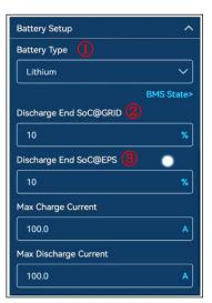
**Notes:** All the settings must be 100% honest to the battery specifications first. Both the two discharge End-up SOC set range is  $10\sim100\%$ .
