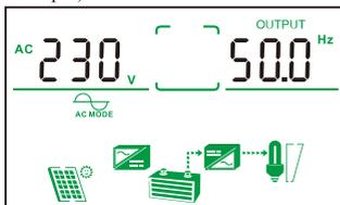
4) Battery working mode (Has PV input but no mains input, only the PV charge the battery)
