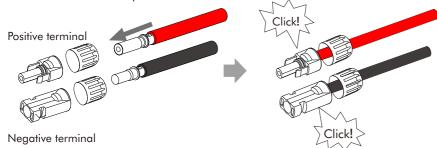
Step 5. Tighten the fastening head and into insert the corresponding positive and negative (PV-/PV+) ports of the inverter.
