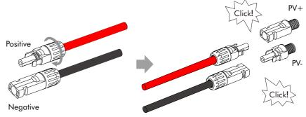
Step 6. Check correct polarity of wire connection from PV modules and PV input connectors. Then, connect positive pole (+) of connection wire to positive pole (+) of PV input connector. Connect negative pole (-) of connection wire to negative pole (-) of PV input connector.
