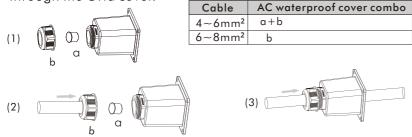
Step3: Remove the cable jacket and strip 70~80mm, And strip wire insulation by 7-10mm.
