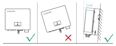
Reserve enough space when installing inverter (at least 300mm) for heat dissipation.
