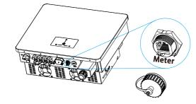
Step 2: Pass the wire harness through the cover with the waterproof plug, and then strip the wire. Stripping requirements: 5-7mm.
