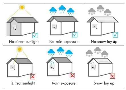
Select an optimal mounting location for safe operation, long service life and expected performance. During the installation and operation process, please the inverter in don't install the inverter where people may touch its casing and radiator, because these parts will be very hot during operation.
