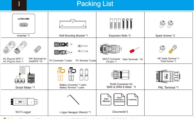
Notice: The number of PV connectorrs/terminals for HP3-5K/6K/8K are 2 pairs, and for HP3-10K/12K are 3 pairs. On receiving the inverter, please check to make sure the packing and all components are not missing or damaged. Please contact your dealer directly for supports if there is any damage or missing components.
