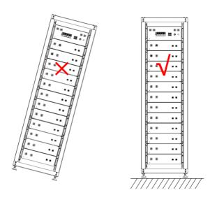
This battery is indoor version and can be only installed in an indoor location. The space around batteries recommended refer to the figure below.
