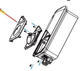
② Step 2: loosen three (for single-phase) or five (for three-phase) screws and one hoop, pass the feeder cable through the charging post feeder sealing ring, and then through the feeder cable hoo
