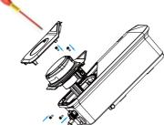
3 Step 3: Insert the cable into the hole before locking, adjust the position of the cable and then tighten the terminals.
